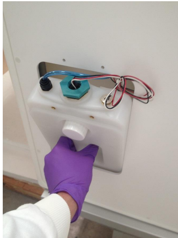
Figure 27: Water Tank tilted forward partially removed
