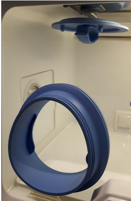
Figure 19: Glove port cap storage location inside workstation
