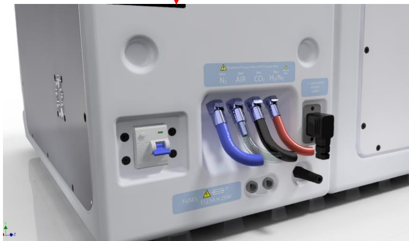
Figure 10: Gas and Electrical Connections
