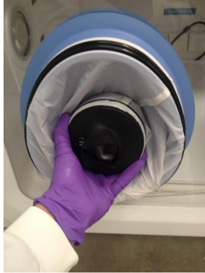
Figure 12: Compressed Ezee-Sleeve for Entry
