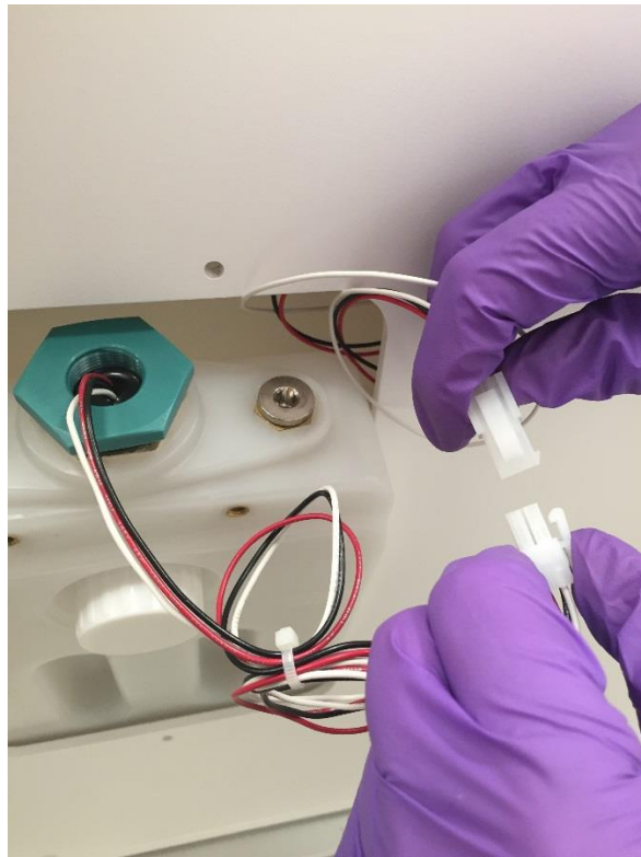
Figure 29: Water Tank electrical connector
