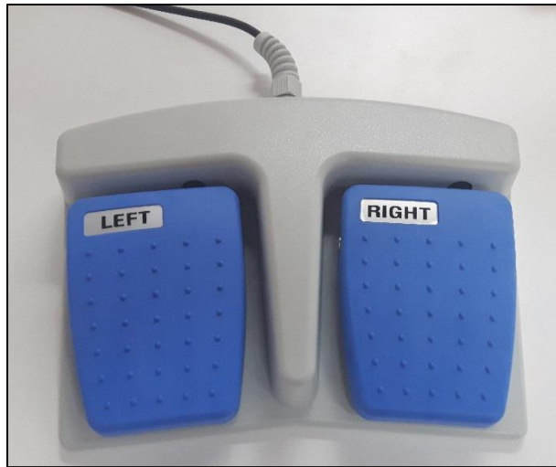
Figure 14: Foot pedals for right and left glove ports
