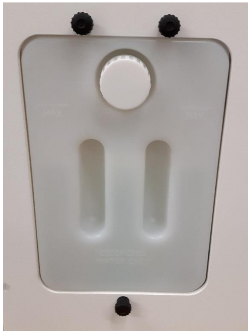
Figure 24: Humidity System Water Tank
