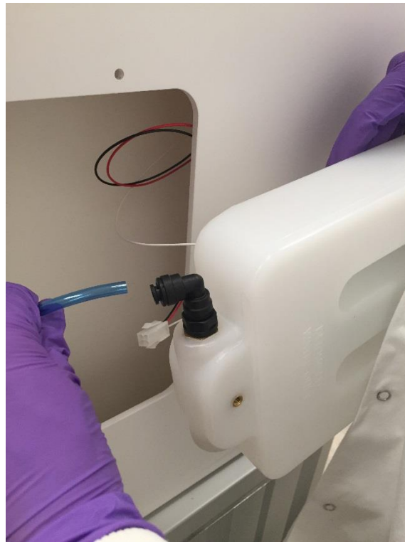
Figure 31: Water Tank bottom tube disconnection
