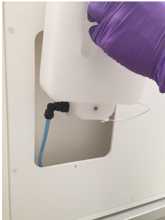
Figure 30: Water Tank bottom lifted out
