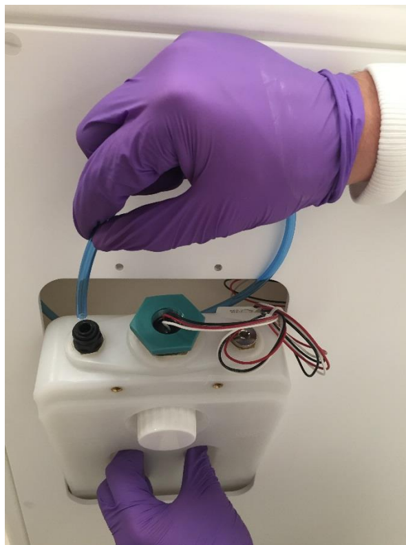
Figure 28: Water Tank top tube removal
